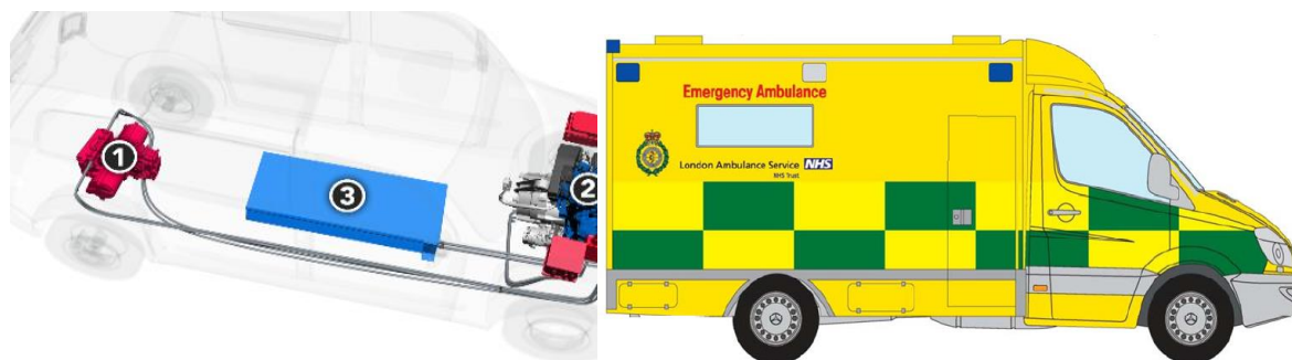
Figure 35: Retro-fit of electric drive to utilise older fleet to extend life and reduce emissions
