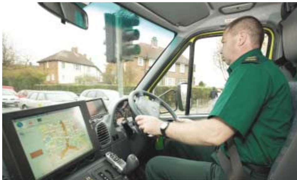
Mobile data terminals allow information about 999 calls to be transferred electronically to vehicles, while satellite navigation guides ambulance staff to the scene using an electronic voice and mapping system
